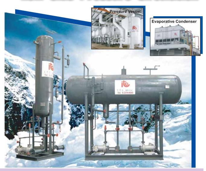
The ITC's Low Side Pressure Separator is a highly specialized design which follows the ASME (American Society of Mechanical Engineers) Section VIII Division 1 requirements. All vessels are made from A516-Gr70 metal sheet (ASTM standard) and can be operated below  $-30^{\circ}$ C. When applied in low side pressure circulation, it can regulate ammonia to be at appropriate level. It consists of 25% of liquid ammonia and 75% free spaces for letting ammonia expand or convert to gaseous form.
