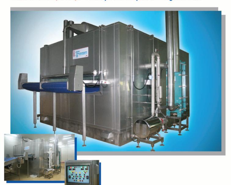
ITC's Eutectic fluid (brine) freezer provides a quick freezing solution for all your product needs. With variable-belt-speed design, a wide range of IQF products can be processed with fast freezing time. The brine freezer ensures less shrinkage, weight loss, and dehydration of your products by using Sodium chloride (NaCl) or Glycol as a freezant that quickly freezes the products in a matter of minutes without causing freezer burns to the texture.
