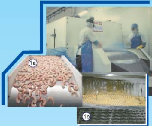
Figure 2a & 2b. An outfeed pathway of Tunnel Freezer (1a.) A cooked peeled shrimp & (1b.) frozen pineapple product
