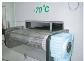
AC variable speed drive gear box with TEFC motor.
