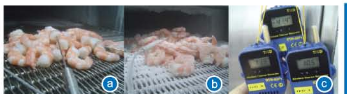
Figure 1 ITC 's testing laboratory a) A cooked peeled shrimp in pre-test freezing b) A cooked peeled shrimp in post-test freezing c) ITC's thermo data logger
