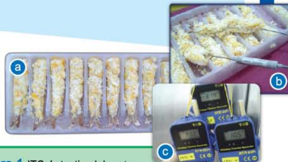
Figure 1 ITC 's testing laboratory a) A breaded shrimp in pre-test freezing b) A breaded shrimp in post-test freezing c) ITC's thermo data logger
