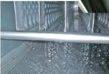
Plate ices falling from plate's sheet surface
