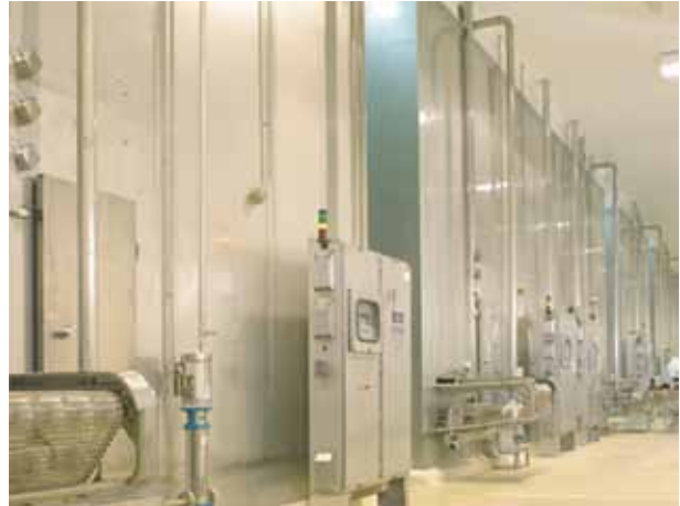
Photo 8 : Totally Welded Stainless Stell Insulated Enclosure Spiral Freezer.
