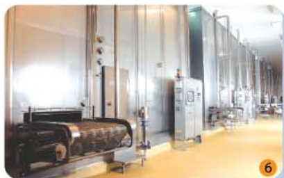
Fully welded stainless steel wall panel enclosure
