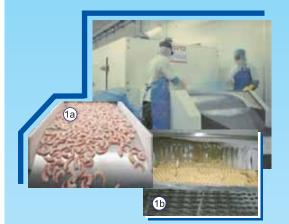
Figure 2a & 2b. An outfeed pathway of **Tunnel Freezer** (1a.) A cooked peeled shrimp & (1b.) frozen pineapple product
