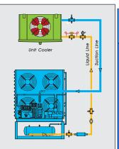
Schematic diagram of the Air Cooled Condensing unit showing connecting lines attached to the unit cooler.
